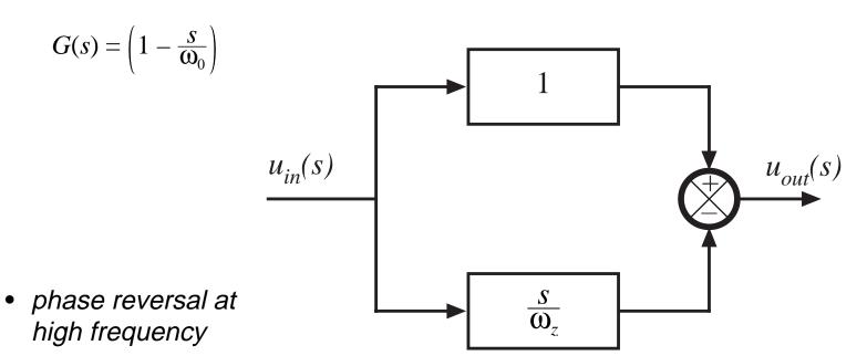
transient response: output initially tends in wrong direction
