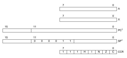
Length depends on the address/memory size of the individual M68HC05, for instance, a 2-K memory map requires an 11-bit program counter and stack pointer as shown. Current length ranges from 11 to 14 bits (2 K to 16 K).
