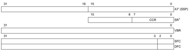
1. The status register (SR) consists of two halves as shown.
