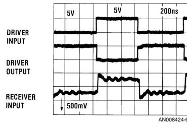
FIGURE 6. A high-speed CMOS device driving another gate through a 28-gauge wire poised above a groundplane ( $Z_0 = 200\Omega$ ) exhibits higher ringing and overshoot than predicted in Figure 5, thus indicating a lower output impedance or higher line impedance than that used in the prediction.
