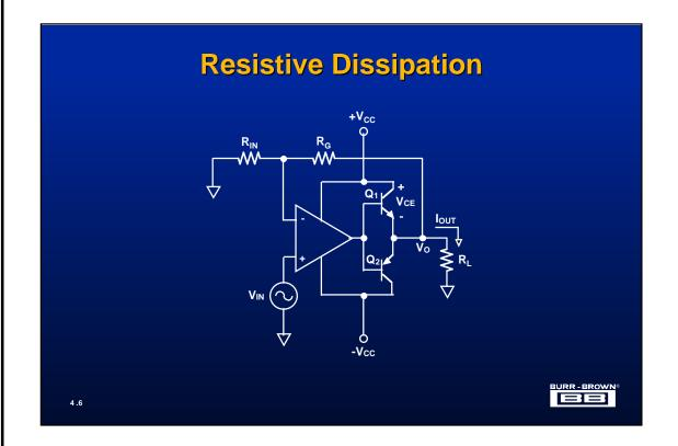
The above diagram shows a simple model of an op amp being driven by an ac signal into a resistive load. The output stage of the POA has been modeled as a pair of transistors. The power dissipated by either  $Q_1$  or  $Q_2$  at any instant is given by the multiplication of  $V_{CE}$  times  $I_{OUT}$ .
