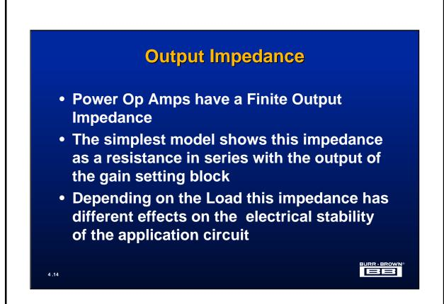
If an op amp had no output impedance, the op amp would be stable under any load conditions. Unfortunately all op amps have some output impedance which has an effect on the stability of the circuitry with respect to load.
