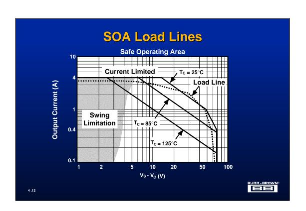
The above graph shows Safe Operating Area or SOA chart for the OPA544. This chart is useful for evaluating the safe electrical and thermal limits of an op amp.
