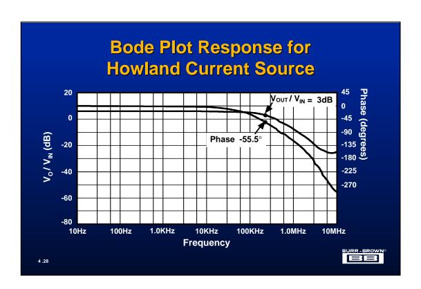
The above graph shows the actual measured closed-loop response of the  $V_{OUT}/V_{IN}$  gain characteristics of the Howland current source.
