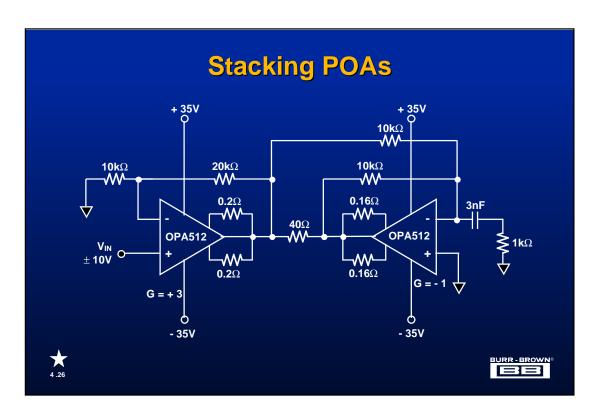
Using a similar master/slave scheme that allows for increasing load current two POAs can be connected as shown above to increase peak-to-peak voltage to a load. The master op amp, on the left, is set for the desired gain and gain polarity while the slave is set for a gain of -1V/V so that its output is the inverse of the master or system gain. This technique not only doubles the available output voltage but also increases the slew rate by a factor of two.
