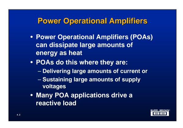
While the great majority of operational amplifier applications are for conditioning small signals and driving high impedances, there are occasions where a low impedance or reactive load is driven or controlled. These are the applications that require a Power Operational Amplifier or POA. A POA is simply an operational amplifier that can deliver large voltages or currents to a load. If the amplifier or load must sustain more than 100mW, the application requires a POA.
