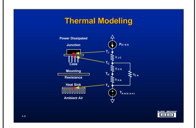
Just because a POA has been selected for an op amp application, that does not ensure it will operate reliably unless a thermal analysis is performed. The data necessary for such an analysis is the thermal resistance of the op amp, the amount of power being dissipated by the amplifier, and the expected maximum ambient temperature.
