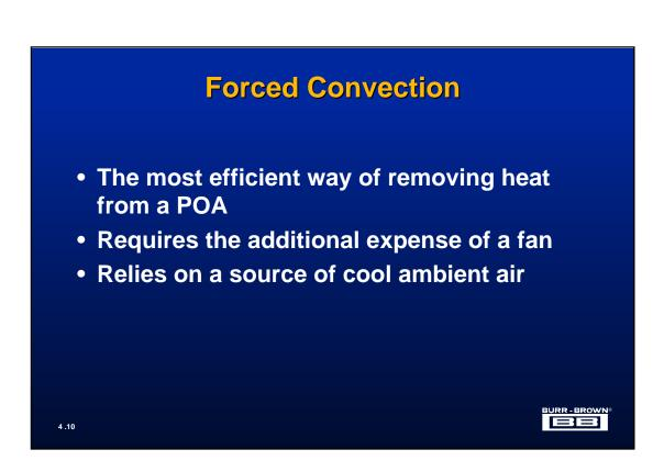
Forced convection is a heat sink with air or liquid from a fan flowing over it. Most data sheets for heat sinks show a graph of the heat sinks  $\theta_{HA}$  versus air flow. Usually this graph is drawn with the units of SCFM for air flow, which stands for Standard Cubic Feet per Minute. SCFM is air flow measured in cubic feet at standard temperature and pressure, i.e. sea level and 25°C. These graphs also go down to zero air flow and this would be the number used with no air flow.
