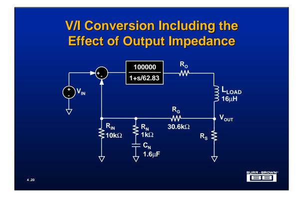
Just as with voltage control of a capacitor, current control of an inductor modifies the apparent open-loop gain of an operational amplifier as seen by the load. Again an additional pole is formed by the reactive load and the output impedance of the amplifier. The apparent open-loop gain of the amplifier is that  $A_{OL}$  curve that we would measure at the point of feedback, in this case the juncture of  $L_{LOAD}$  and  $R_{S}$ .
