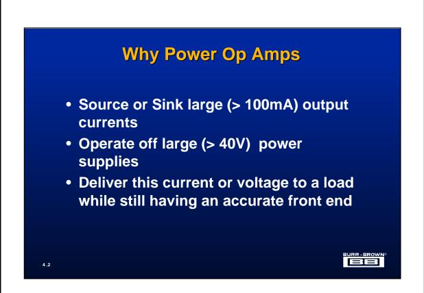
The simplest way to envision a Power-Operational amplifier is to think of it as a conventional op amp built with high voltage transistors and physically large output devices. In fact, some of the earliest power operational amplifiers were built by combining a high voltage, low current op amp with an output stage made from high current darlington transistors.
