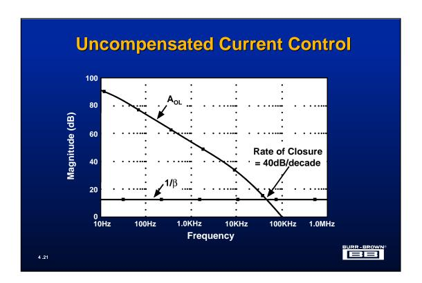
The above plot shows the intersection of the modified open-loop gain characteristic of the current controlled inductor and its  $1/\beta$  plot. As was seen with the uncompensated voltage amplifier, when driving a capacitive load, the rate of closure is 40dB/decade and this circuit is unstable.
