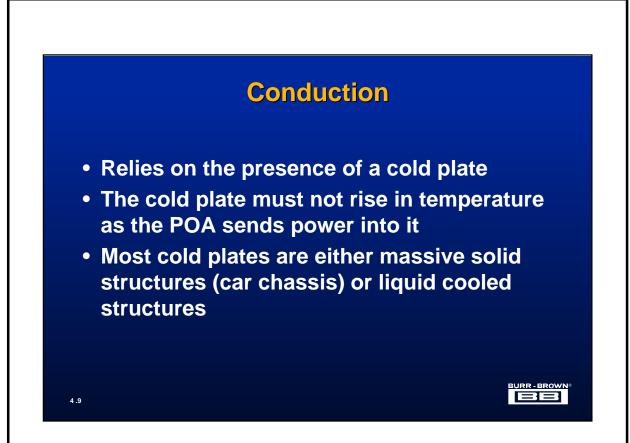
If the system that the POA is being used in has a solid continuous temperature body, the dissipated power from the op amp can be moved to this body. This cool body is sometimes referred to as a cool plate. For example, the chassis of a car or airplane could be a cool plate if the chassis is sufficiently large. Of course, the power being added to the chassis would increase its temperature if the power was not removed by another heat removal method, usually convection.
