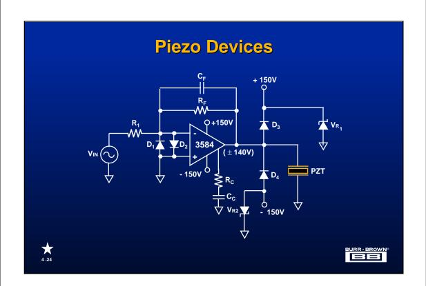
Piezo transducers are used for micro-positioning functions found in surface profiler, scanning tunneling microscopes, and mirror positioning for laser applications.
