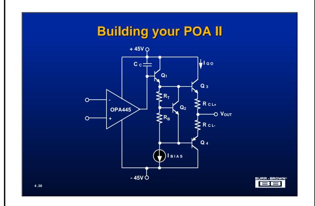
Solving the cross-over distortion problem of the previous circuit can be done with the addition of a class A-B output stage to the OPA445.
