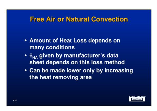
Free air or natural convection is the most common way that electronic devices shed energy as heat. This is also the method that all heat sinks work when not in the presence of forced air i.e. a fan.
