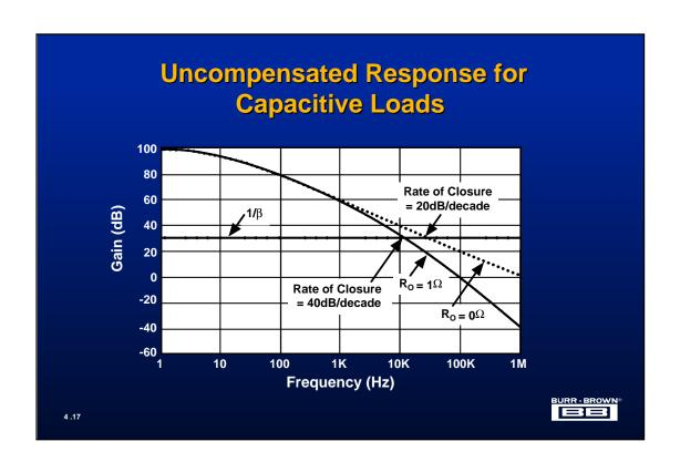
A well known test for the stability of an operational amplifier is to plot the inverse of the feedback factor  $\beta$  versus frequency on the same graph as the apparent open-loop gain curve of the amplifier in use.
