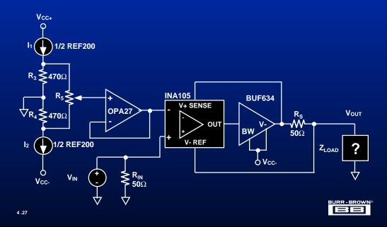
Another application for a POA is the conversion of voltage into an equivalent current. Quite commonly this converted current is used to drive a reactive load. If a POA was used in this configuration with discrete resistors it would be quite common to have stability and accuracy problems. The accuracy problem could be solved with expensive matched resistors. The stability problems could be overcome by noise gain compensation.
