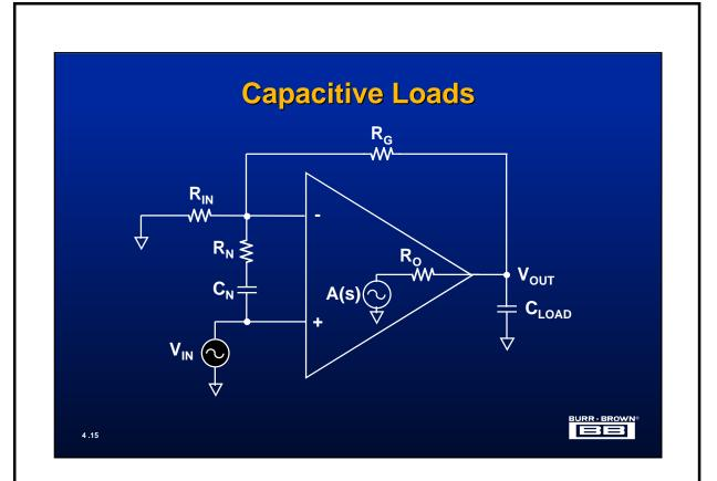
The above diagram shows the pertinent circuit elements used to evaluate the performance of the op amp when presented with a capacitive load. The output impedance has been modeled as simply a resistance of constant value,  $R_0$ . While most output impedances also have a reactive element associated with this resistance, it is usually not necessary to include this for a successful stability analysis.
