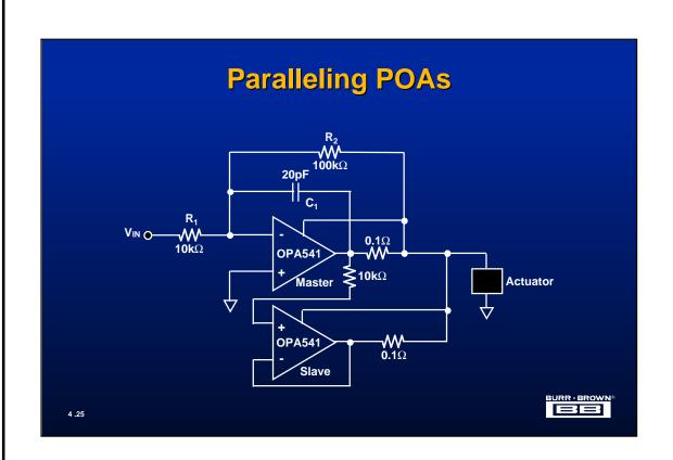
One of the more common application problems that come up when selecting a Power Op Amp is that the manufacturers line does not offer a device that has sufficient current for the application. It is possible using the scheme shown above to parallel like op amps for more output current.
