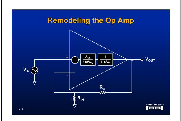
The above diagram shows a first order model of the power operational amplifier which includes the effect of output impedance as it reacts with a capacitive load.
