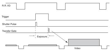
This is an excellent application for capturing multiple images (two fields of images) of indexing objects under various lighting or brightness conditions. When frame mode is selected, the full vertical resolution is achieved even when using an electronic shutter by taking two fields of shutter images.
