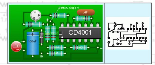
I installed this circuit in my S10 Chev 1990 pickup, right into the headlight switch compartment. The battery 12 V supply is always hot on the switch terminal and Ground should also be available. Make your Circuit small enough to fit well into the space where it will be installed. I drilled a small hole on the face plate and installed the LED (red, and the brightest available).
