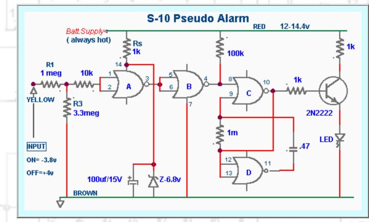
The circuit is simply a low voltage detector created by putting together a CD4001(A&B), an oscillator(C&D) driving a 2N2222 transistor, and an LED. The CD4001 gates have a threshold voltage of 3.4V, the sensitivity input is 1Mohm/V. Voltage input must be greater than the nominal 3.4V.
