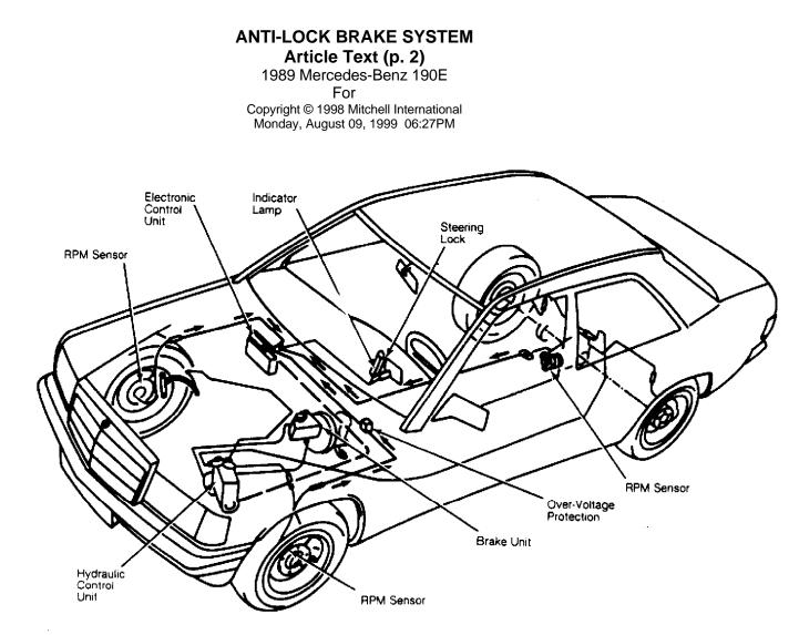
Fig. 1: Mercedes-Benz ABS Component Location Courtesy of Mercedes-Benz of North America.
