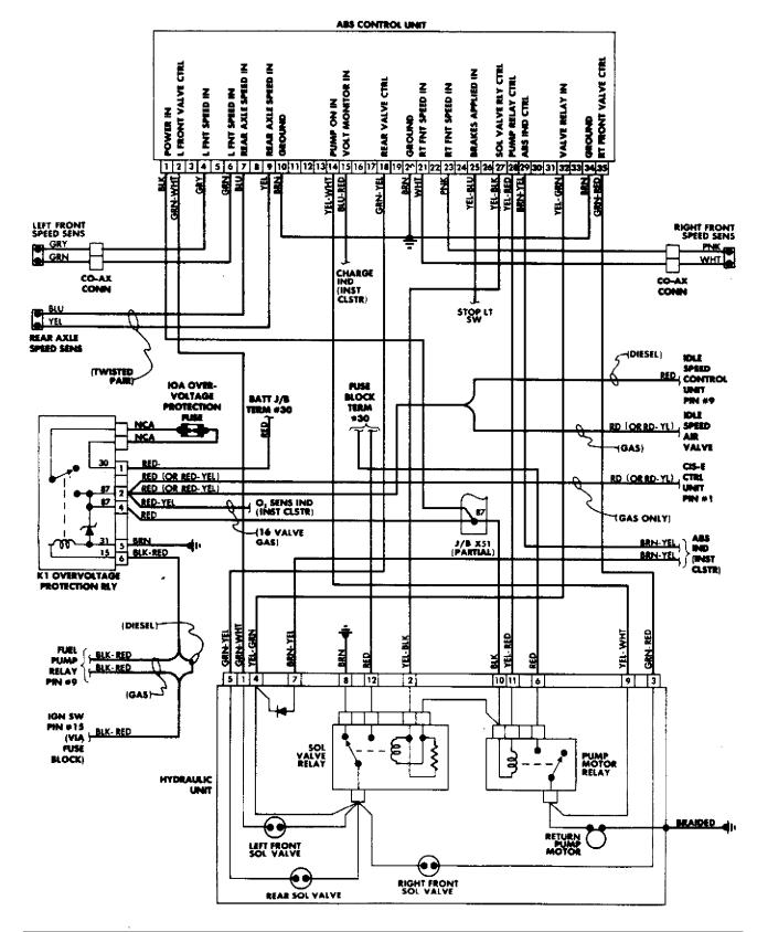
Fig. 4: Mercedes-Benz 190E Anti-Lock Brake System Wiring Diagram
