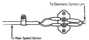
Fig. 3: Rear Speed Sensor Harness Connector (Under Rear Seat) Courtesy of Mercedes-Benz of North America.
