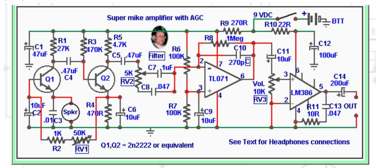
When RV1 resistance is high C1 time constant is low ( slow discharge ) and allows lower frequencies which have a higher signal amplitude to be amplified and when RV1 is set to its lower resistance setting limited by R2, C1 discharge very fast allowing only higher frequencies to be amplified, thus we have frequency filtering and automatic gain control. Please note that R1 and R4 values are critical and must not be changed for the AGC to work as designed.
