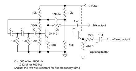
Adjust the 68 ohm resistor for lower distortion if desired and vary one of the 1N914's 10k divider resistors to adjust the output amplitude. The optional buffer will drive low resistance loads and provides load stability.
