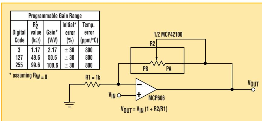
1. The thermal performance of a simple gain circuit using a digital potentiometer in this configuration is typically 800 ppm/°C.
