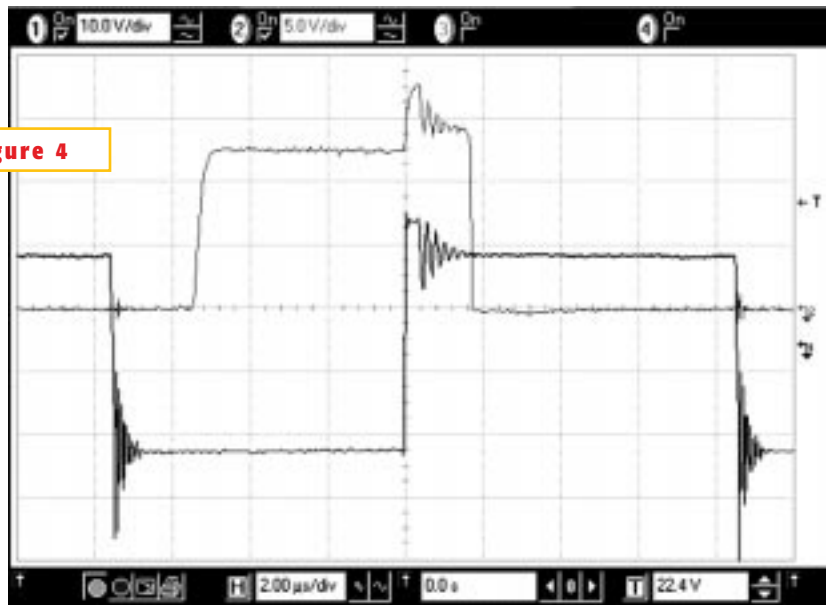
By delaying the sampling time, you obtain a clean auxiliary level that is devoid of any leakage-inductance effects.
