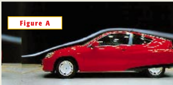
The abrupt Kamm back at the rear of Honda’s Insight ensures clean airflow separation for constant aerodynamic forces on the car.
