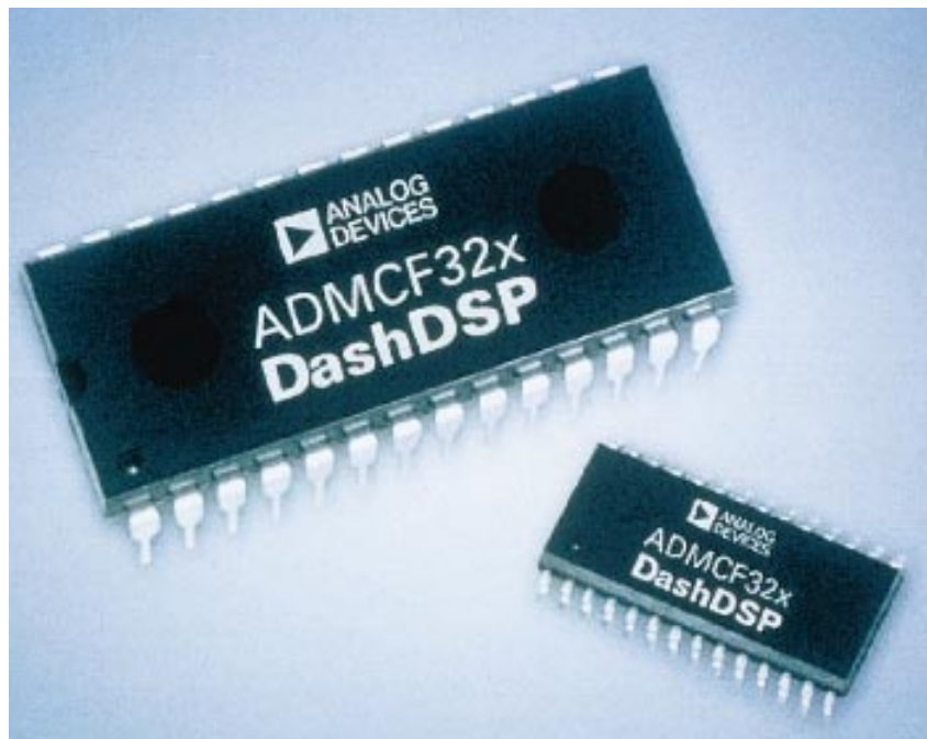
A family of DSP motor-control ICs from Analog Devices incorporates flash memory.
