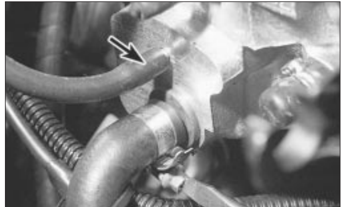
16.6 Slackening coolant hose retaining clip from front of inlet manifold - MAP sensor hose arrowed
