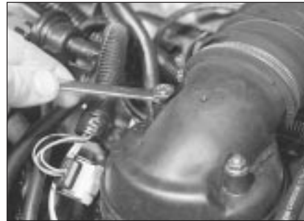
12.1a Undo the two nuts . . .
