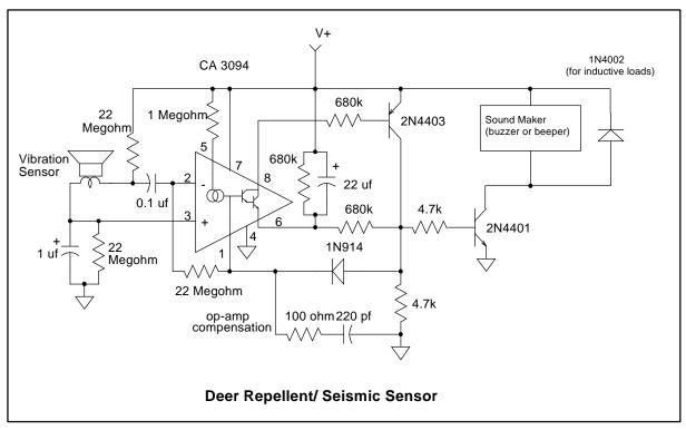
The unit is designed to consume minute amounts of power when not rattling to provide many months of unattended protection (practically set by the battery shelf life). The seismic sensor is built from an ordinary 2 inch speaker by gluing a mass to the speaker cone to lower its resonance frequency. A lid from a baby food jar with a little extra weight glued to the inside will work fine.
