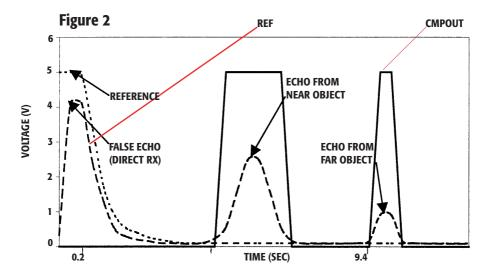
By comparing the ECHO and REF signals, the range-finder circuit effectively inhibits the large-amplitude receive signal at time t=0.2 msec.
