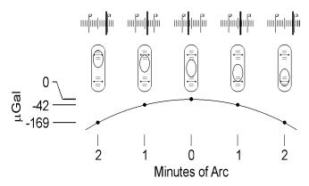
If the meter is nulled to the reading line when the meter is out of level, the gravity reading will be less and less the more the meter is out of level. Be sure the other level, the long or longitudinal level, is in the level position each time the meter is read.
