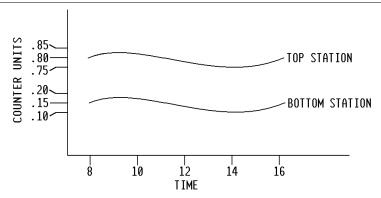
The separation between the two curves is the average counter reading difference  $\Delta\,C$
