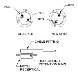
The new Mark power fitting can be recognized by the orientation key being on the top and the power pins being 90° from the direction of the cable. Also, there is a half-round groove just inside the socket that accepts a half-round protrusion on the molded cable fitting at the meter end of the power cable. The new Mark fitting solved a serious drawback of the older fitting. The new fitting has
