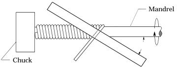
Another method is to hold the wire at an angle and with tension while winding it on a rotating mandrel.
