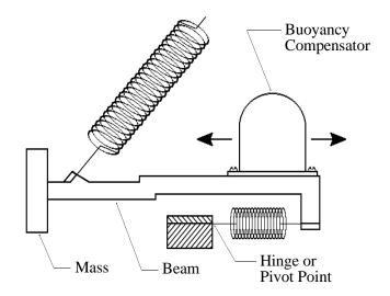
If the sensor develops a leak, The compensator will allow an accuracy as good as other gravity meters in good working order. However, the accuracy will be less than optimal and less than desired for careful gravity observations.
