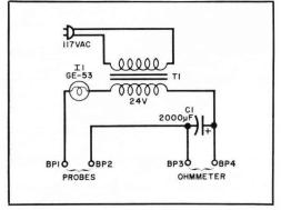
Simple survey meter circuit can be easily assembled in a utility chassis.
