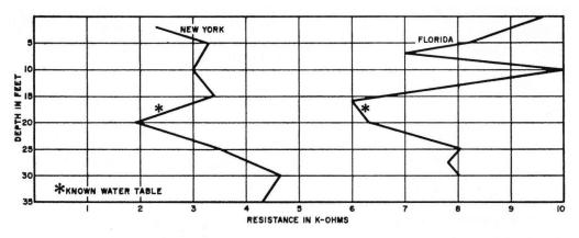
Two test recordings made in widely separated localities show striking similarities in that the resistance drops appreciably at depths where known water tables exist.
