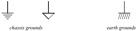
FIGURE 1.2. Symbols used for ground in circuits.
