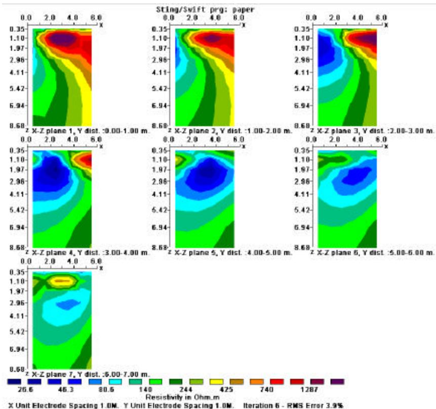
Figure 6 – 3-D Electrical Imaging model showing vertical slices in the X-Z plane for Case #2.
