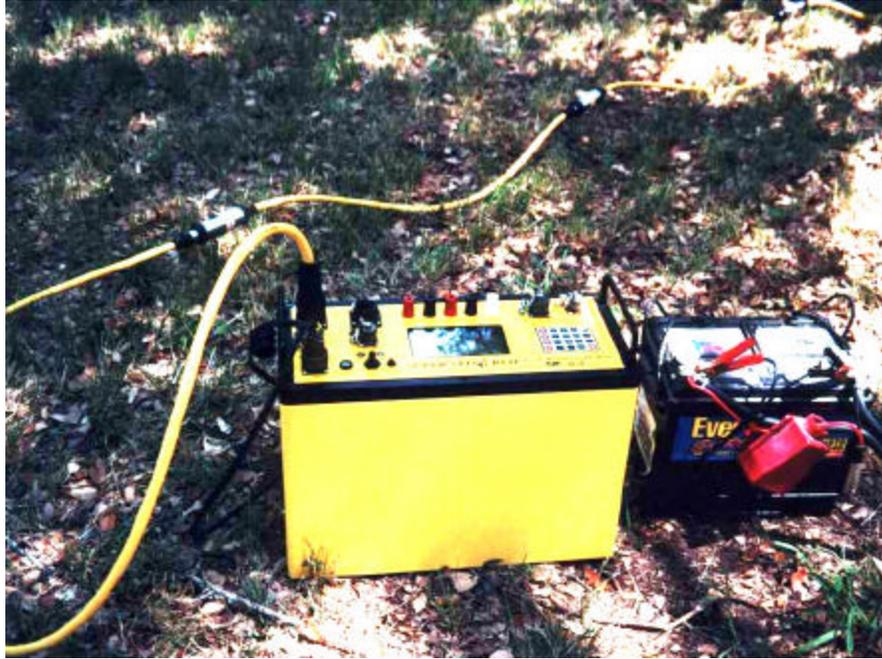
*Figure 10 – New SuperSting R8 IP EI System manufactured by AGI.*
