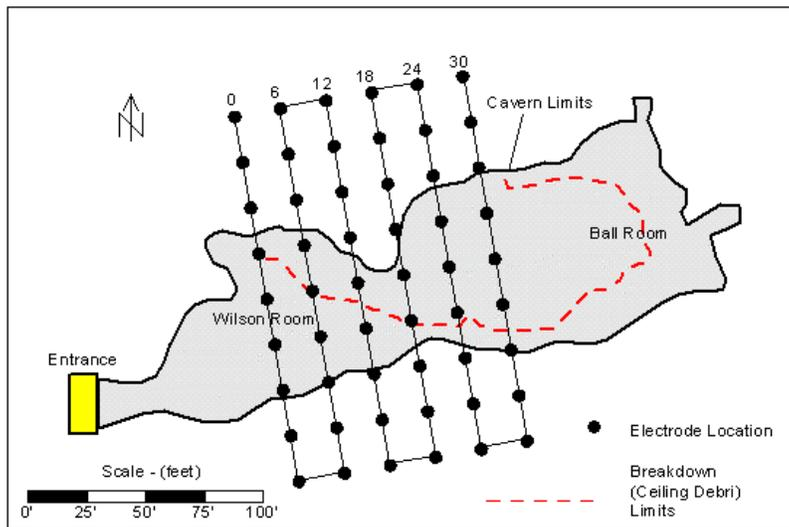
Figure 2 - 3-D Electrical Imaging survey grid over Indian Echo Caverns (Courtesy of SAIC).
