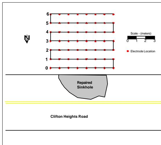
Figure 5- 3-D Electrical Imaging survey grid adjacent to the Clifton Heights sinkhole.
