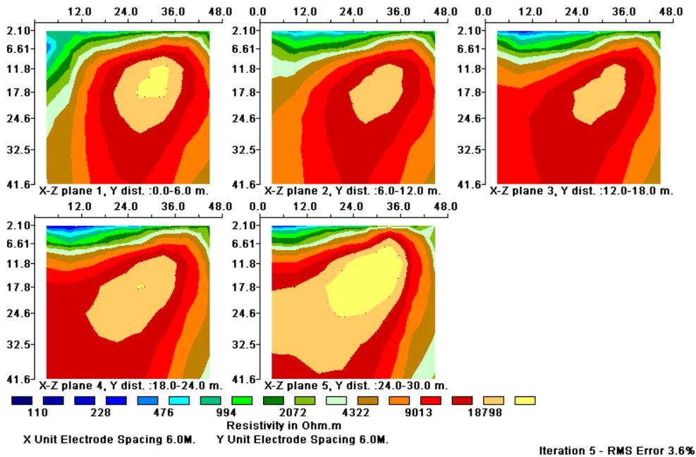
Figure 3- 3-D Electrical Imaging model showing vertical slices in the X-Z plane (Courtesy of SAIC).
