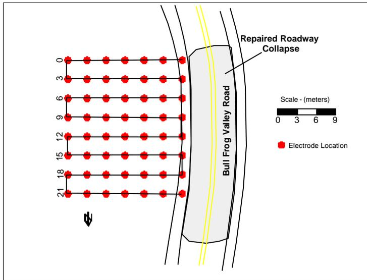
Figure 8- 3-D Electrical Imaging survey grid adjacent to the Bull Frog Valley Road sinkhole in Case History #3.
