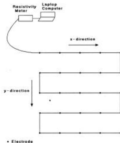
Figure 1. A schematic diagram for one possible layout for a 3-D survey (Loke, 1997).
