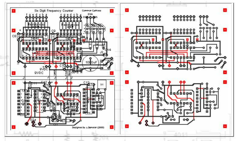
• For the experienced hobbyists point to point wiring is quite possible using No 24 and smaller gauge wire, for a single layer board it is essential that all jumpers shown in red be installed before parts and sockets are soldered into place. For jumpers under the socket I use bared wrapping wire inserted in the wholes leaving about 1/4 " of wire produting on the solder side then fit the sockets into place then soldered all points.
