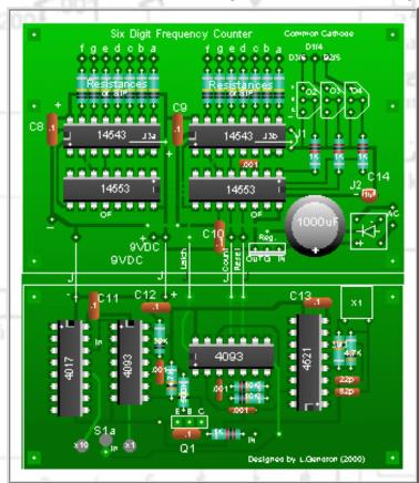
The upper part is the digital display circuitry and the lower part is the input and signal conditioning.
