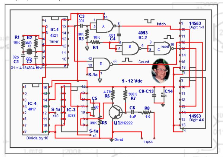
To obtain a count of more than 1 MHz, IC-4 CMOS 4017 is added to enable us to count up to 12 MHz which is the maximum operating frequency of IC-4. The output of IC-3 from pin 11 is also sent to IC-4 pin 14, IC-4 is used as a frequency divider and is configured to divide any frequency by 10, thus for a given frequency of 10 MHz the counter will register and display 100,000.
