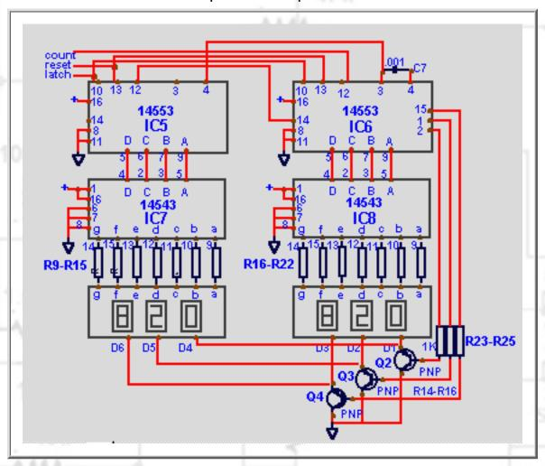
To display six (6) digit we simply add an exact duplicate of the three digit circuit and connect the overflow from pin 14 of IC-6 to pin 12 of IC-5 as well as carry the oscillator signal from pin 3 of IC-6 to pin 4 of IC-5 and duplicate the inputs of the "
