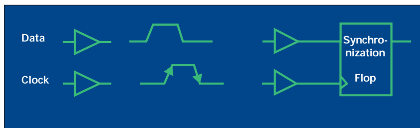
Figure 1. Double data rate interfaces transmit data on both edges of the transmit clock.
