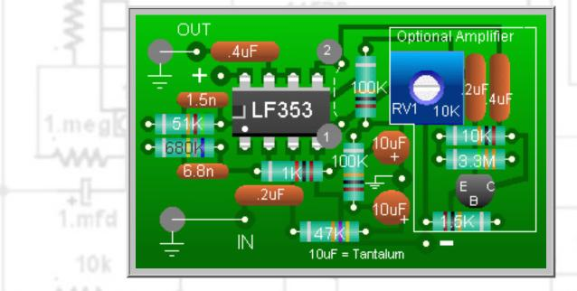
The layout is for a single channel pre-amp. Duplicate the circuit layout or PCB for Stereo, connect positive, negative and ground points together. Use stereo input and output plugs and shielded wire . Ensure that all grounds and wire shields (mesh) are connected to Ground of the circuit . It is also recommended that a metal enclosure be used to minimize noise and Hum .
