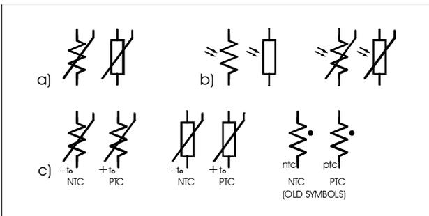
*Fig. 1. Typical sensor resistor symbols (a) voltage dependent (VDR or varistor); (b) light dependent (LDR); (c) thermistor. Symbols may be enclosed in circles or ovals. These symbols should not be confused with those in 3/3.2 Fig. 1.*
