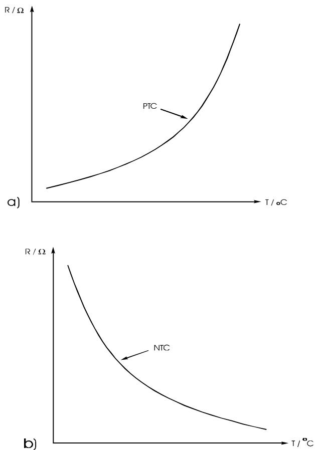
*Fig.4. Characteristic curves for (a) PTC thermistor and (b) NTC thermistor.*
