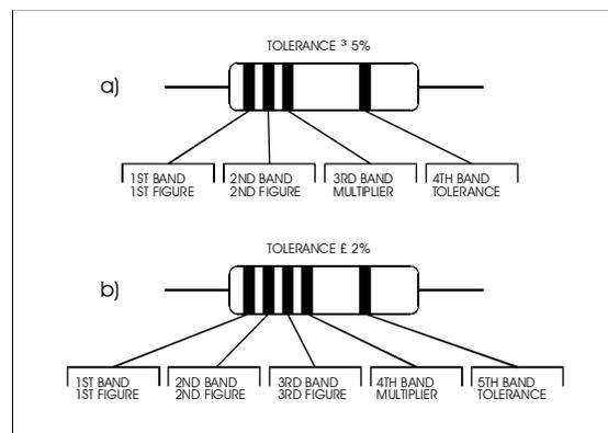
Fig.2. Resistor color code bands
