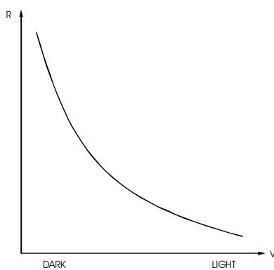
*Fig.5. Characteristic curve for a light dependent resistor (LDR).*
