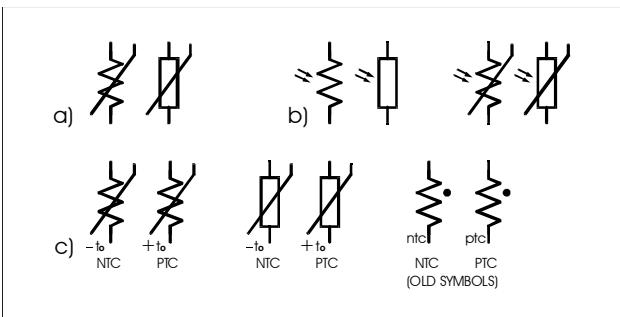
*Fig.1. Typical sensor resistor symbols (a) voltage dependent (VDR or varistor); (b) light dependent (LDR); (c) thermistor. Symbols may be enclosed in circles or ovals. These symbols should not be confused with those in 3/3.2 Fig.1.*
