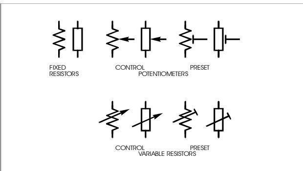
*Fig.1. Typical resistance symbols (see also sensor resistor symbols in 3/3.3 Fig.1)*
