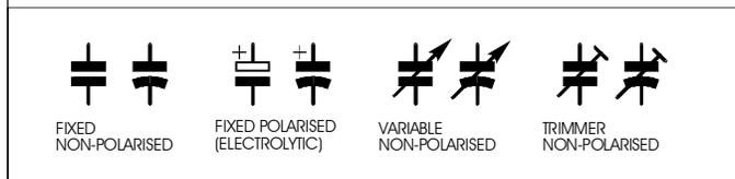
Fig1. Typical capacitor symbols
