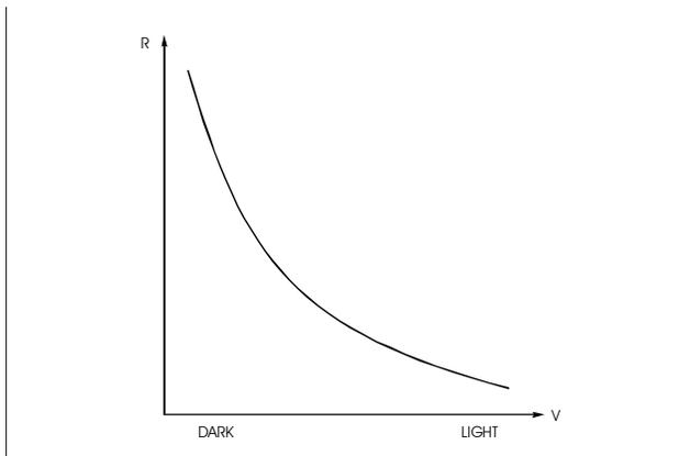
Fig.5. Characteristic curve for a light dependent resistor (LDR).
