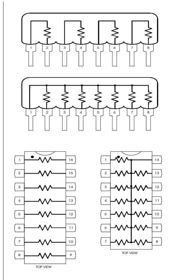
Fig.3. Examples of fixed resistor modules.
