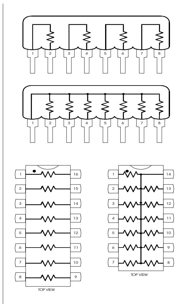
Fig.3. Examples of fixed resistor modules.
