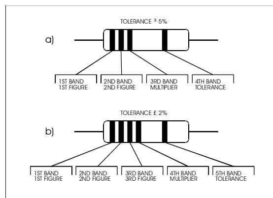
*Fig.2. Resistor color code bands*
