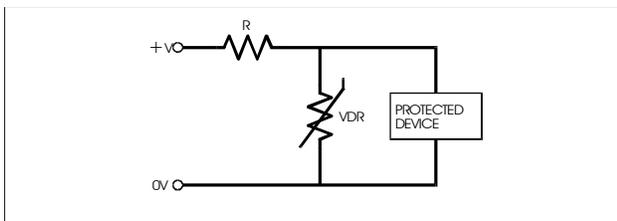
Fig.3. Using a VDR to protect a circuit device.
