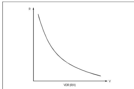
*Fig. 2. Characteristic curve of a voltage dependent resistor.*
