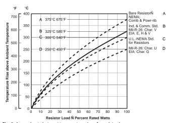
Fig. 2: Approximate hot spot temperature rise of a resistor in free air for various specifications.
