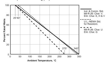
Fig. 3: Derating for ambient temperature.
