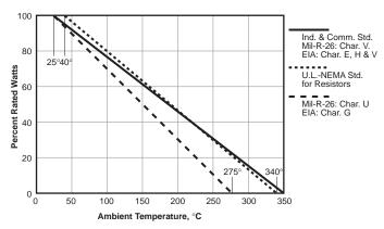
Fig. 4: Derating of Resistors for High Ambient Temperatures.
