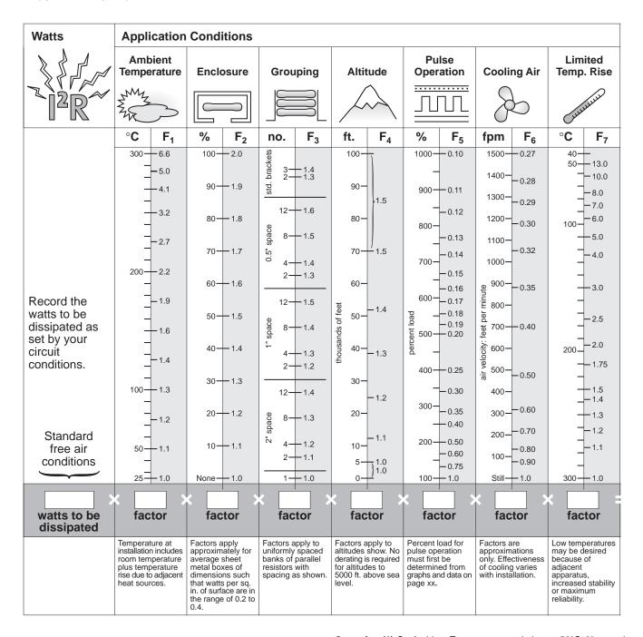
Example: Four resistors, each dissipating 115 watts, are to be mounted in a group. Spacing is to be 2" surface to surface. Ambient to be 50°C (122°F). Enclosure to be total. Other factors standard. Determine Watt
