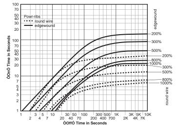
Fig. 13: Percent of Continuous Duty Rating for Pulse Operation of Powr-Rib®,
