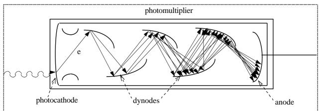
A photon passes through the transparent glass window, and liberates an electron from the alkali metal cathode (such as a Caesium-Rubidium mixture) deposited on the inner surface of the glass. The quantum efficiency of this process (the probability of liberating an electron per photon) is typically 20 to 25%.
