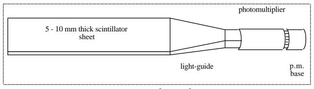
The scintillator may have an area of a few  $cm^2$  to  $\sim 1 m^2$ , depending on the application. Light travels along the thin sheet undergoing many total internal reflections. Most light travels close to the critical angle, and the surfaces must be highly polished to avoid losses.
