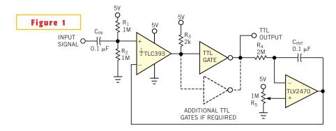
You can obtain a square wave with 2 to 98% duty cycle with this simple circuit.
