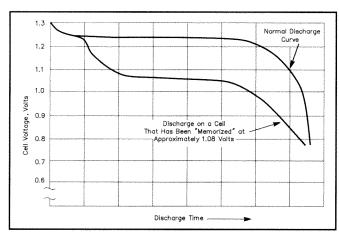
Figure 1—Discharge characteristics of a normal NiCd versus a cell with memory effect.
