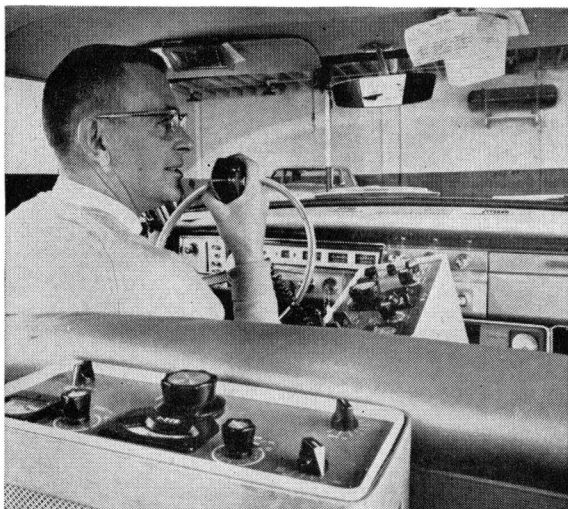
The author in the special car fitted out by the Southern California Edison Company for hunting sources of radio noise. Complete receiving coverage from the broadcast band through 2 meters, plus ham-band transmitters, makes this a really complete mobile station.
