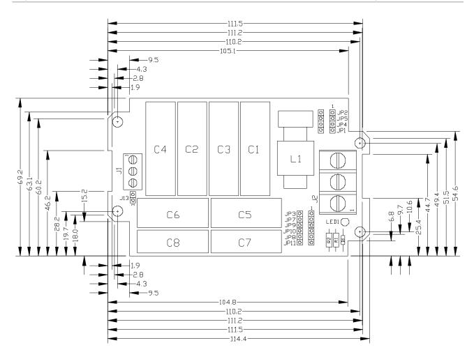
Figure 8: Mechanical Dimensions Antenna Tuning Board
