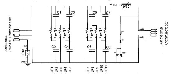
Figure 6: Antenna Tuning Board Schematic
