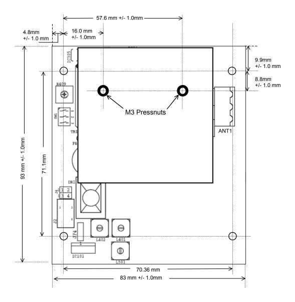
Figure 7: Mechanical Dimensions RA-RFM
