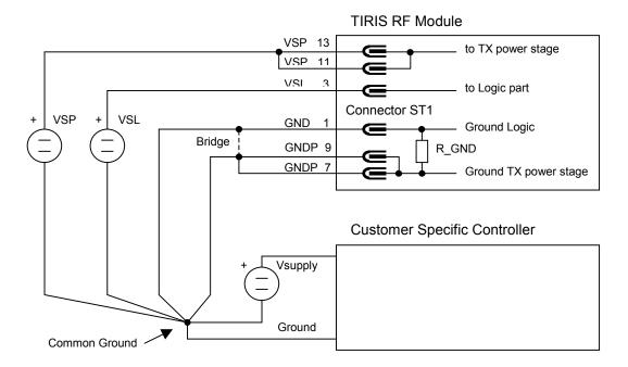
Figure 9: External Ground Connection (GND to GNDP)
