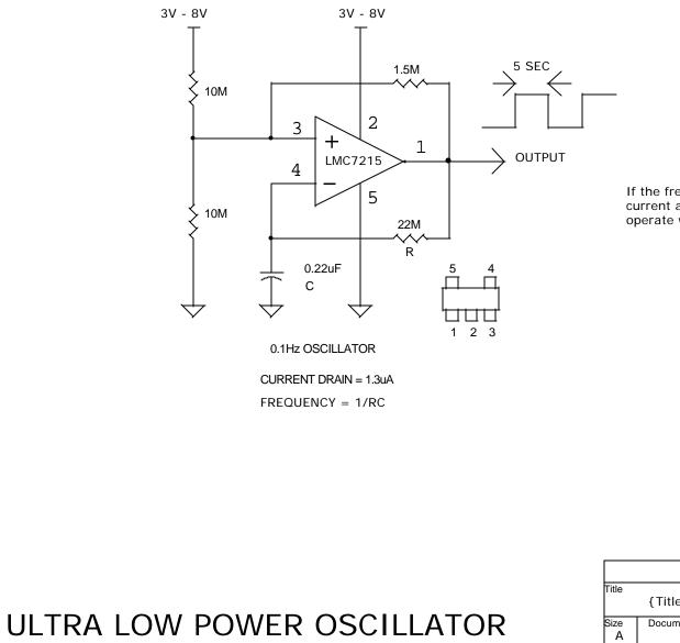
If the frequency and the output drive current are kept low, this circuit will operate with DC supplies below 1.5v.
