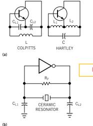
A ceramic resonator (b) takes the place of the inductors in the LC oscillators (a).
