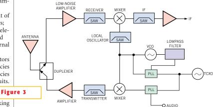
A typical cellular application uses as many as four SAW bandpass filters.
