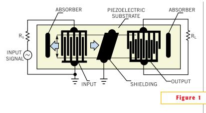
A SAW device works by "acoustic" propagation through a ceramic medium.
