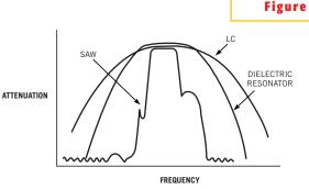
A SAW bandpass filter has much steeper skirts than an LC or a dielectric-resonator filter.
