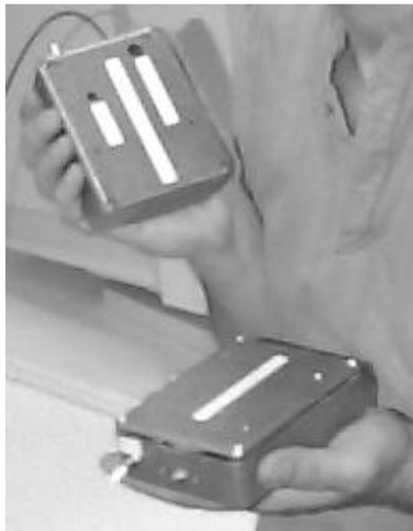
**Figure 8. PAN receiver (left) and PAN transmitter (right). The case and aluminized mylar mounted below the case are receiver electrodes. The transmitter lid and case are**
